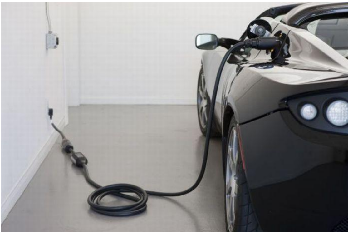
Figure 44: Electric Vehicle Using Standard 10 Amp Power Socket (2010 Dewhurst Photography)
