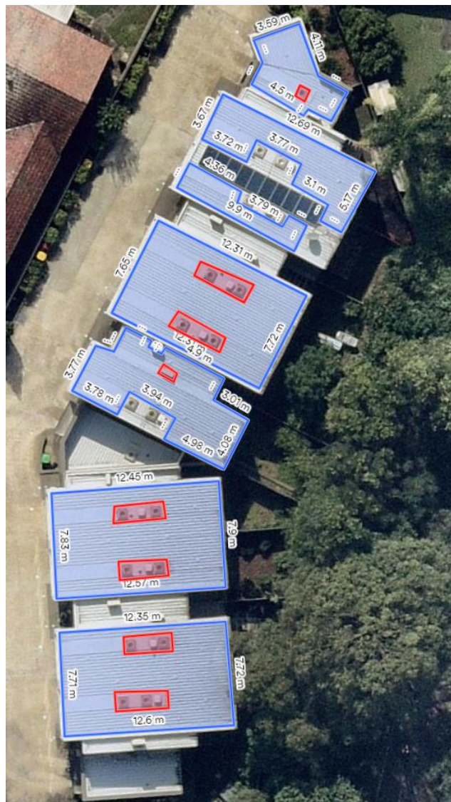
Figure 2: Available roof space to be used for solar at 6 Noel Street, Adamstown
