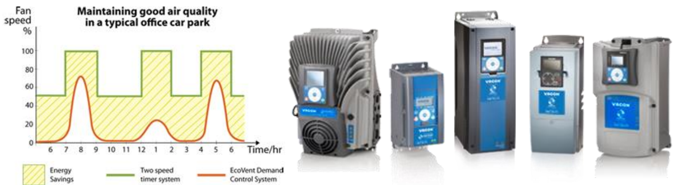
Fig. 16 From left to right, Energy savings from VSD demand control vs two speed fans, Examples of Fantech VSDs
