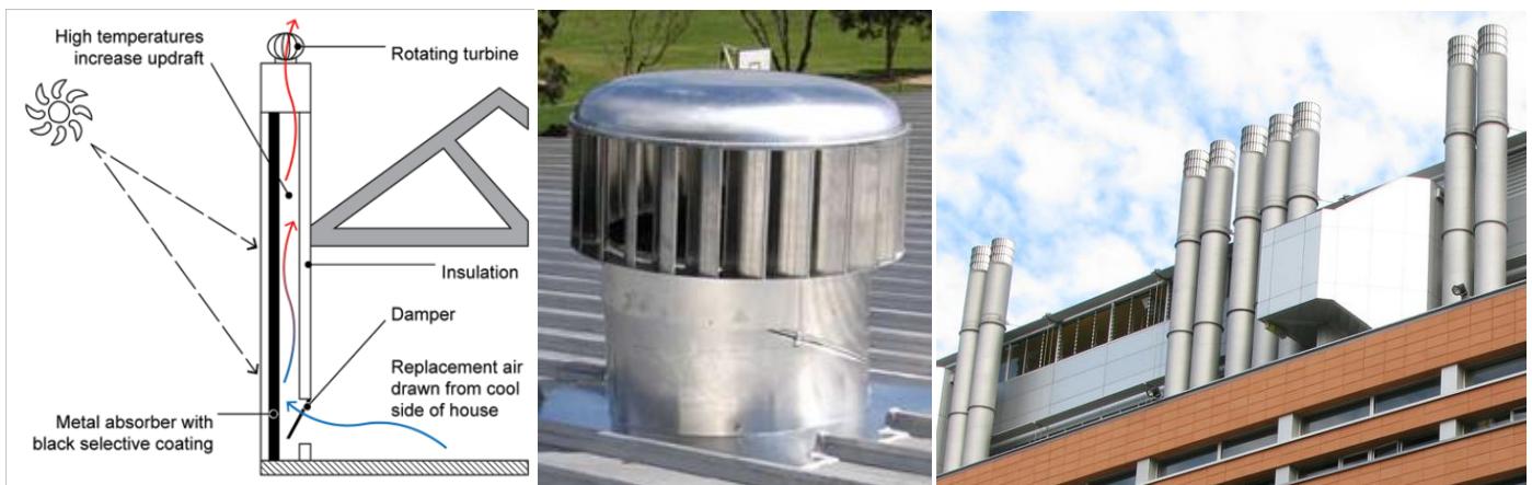
Fig. 18 Passive Ventilation Principles, Small Thermal Flue, Large Thermal Flues at UNSW Red Center
